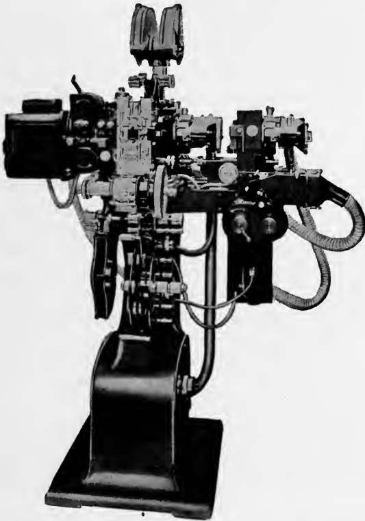
FIG. 16. Debie Matipo TU printer; this printer prints picture, sound-track, and superimposed titles in one operation. Only a single frame of film area is used for each title negative. Insertion of titles and light-changes is fully automatic.
